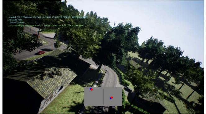
Fig. 1: The 3DC-VO network architecture can be trained to regress scale-accurate odometry information from video data. Shown above is a screen capture from a quadrotor simulator with superimposed predicted (red) and ground truth (blue) joystick positions. Joystick positions are equivalent to thrust (acceleration) and angular velocity of the quadrotor.
